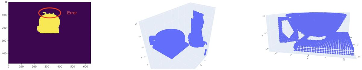
Fig. 8: Errors in the edges of the segmentation map (left) can lead to failures in the unprojected point cloud (middle). We thus use statistical outlier removal to remove outliers from our perception maps to get our crops (right)
